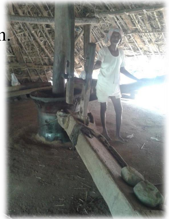
Ghani expeller (traditional cold pressed oil extracting unit) at Kothavalasa, Visakhapatnam, Andhra Pradesh
