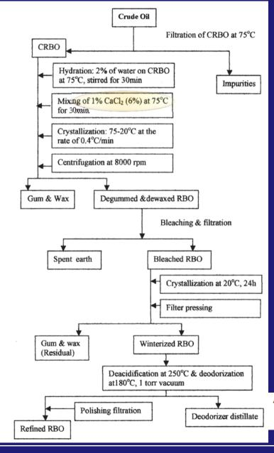
Combining degum / dewax at cold conditions can solidify and remove most of the wax together with the gum fraction in a HSS. Increased viscosity and thus higher oil loss (if pH neutral water degumming). pH-neutral cold degumming (a la the Unilever seed oil Unidegumming) might provide sufficiently low gum levels (5 ppm P). The effect of added CaCl<sub>2</sub> is not explained (could be emulsion breaking electrolyte).
