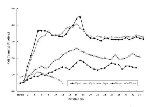
Fig. 4. Performance of *Dunaliella salina* (Australian) cultured at 18x10<sup>3</sup> lux and at different high salinities (50 to 250 psu).
