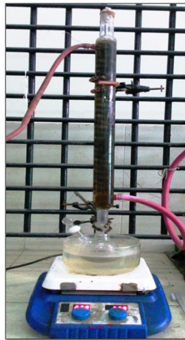
Fig 5: Biodiesel production using heterogenous catalyst.
