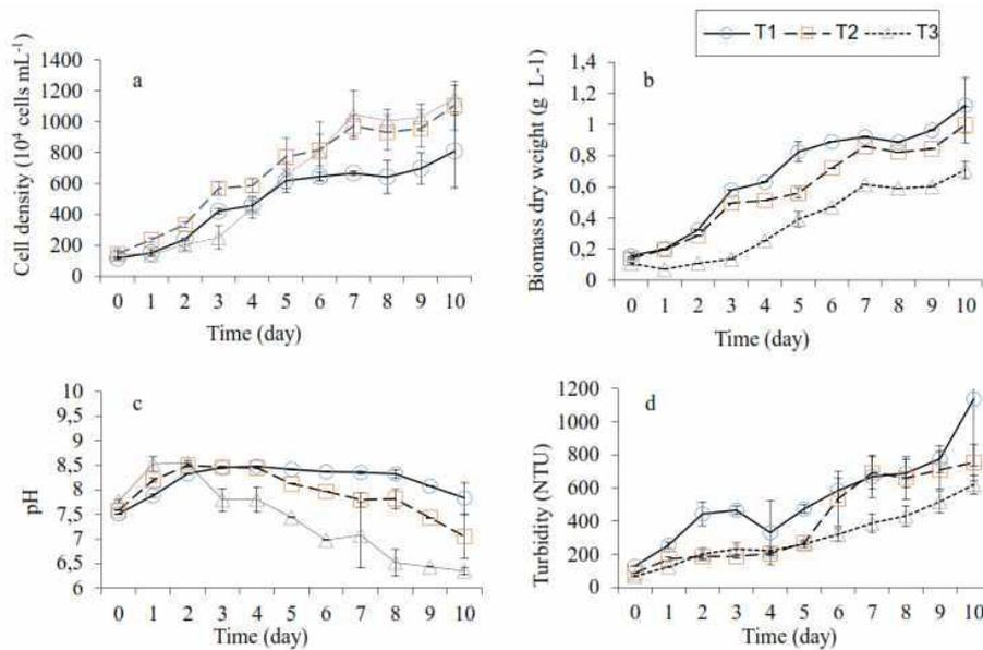
Figure 1. (a) Cell density variation ( $10^4$  cells  $\text{mL}^{-1}$ ) during cultivation period. (b) Dry biomass variation ( $\text{g L}^{-1}$ ) during cultivation period. (c) pH variation during cultivation period. (d) Variation of turbidity in nephelometric units during the cultivation period. Each line refers to the average of four replicates of each experimental treatment. T1 - TAP Medium; T2 - 50% Wastewater; T3 - 100% Wastewater.
