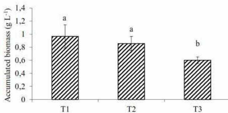
Figure 2. Accumulated biomass during cultivation period ( $\text{g L}^{-1}$ ). Each bar refers to the average of four replicates of each treatment. T1 - TAP Medium; T2 - 50% Wastewater; T3 - 100% Wastewater. Different lowercase letters represent significant differences ( $p < 0.05$ ).
