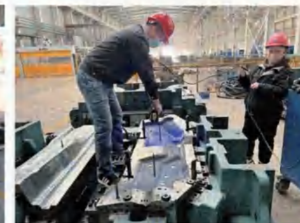
Handy ATOS to scan die 3D cut quality in CNC
