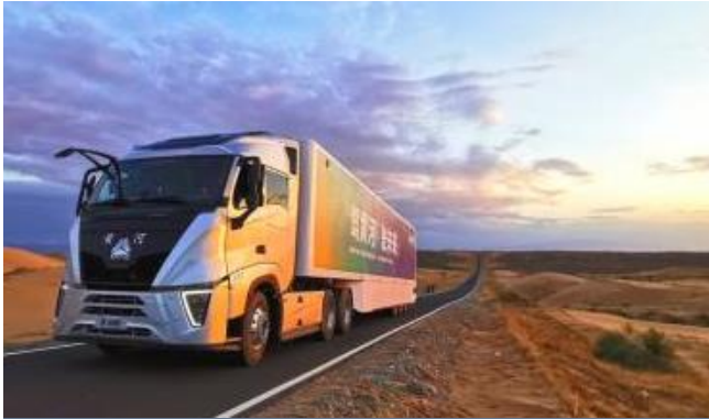
全球首款风阻系数0.37的全新一代高端黄河重卡 Yellow River new generation of heavy duty truck with a wind resistance coefficient of 0.37
