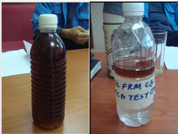
Figure 12: Physical Test for Presence of Polychlorinated Biphenyls (PCB) in Transformer Cooling Oil
