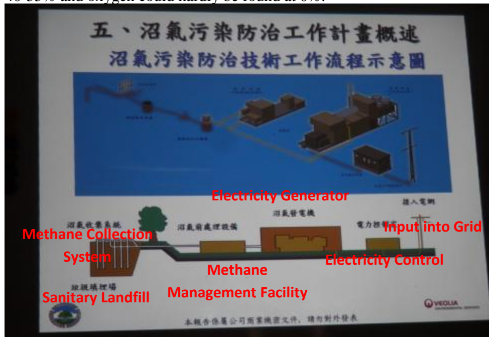
Figure 32: Methane Gas Power Plant Overview
