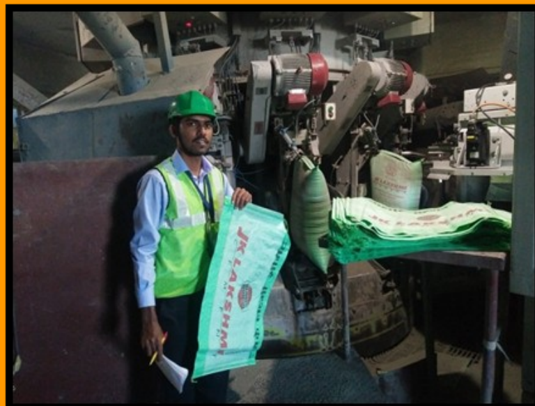
Polypropylene bags that are used to pack cement at Auto Bag Placer Machine
