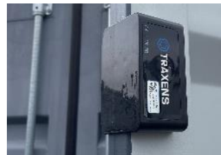
Removable tracker , snapped to the door thanks to its magnet.
