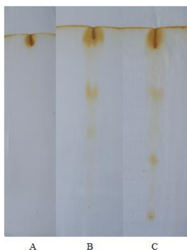
Fig. 4 Thin layer chromatogram of phosphoglycolipids extracted from three algae studied. A- Spirogyra neglecta , B- Pithophora oedogonia , C- Microspora indica .
