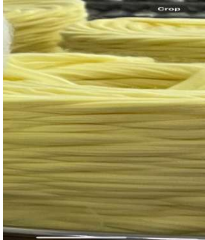
P-aramid 1.45 g/cm 3 Highly crystalline in nature
