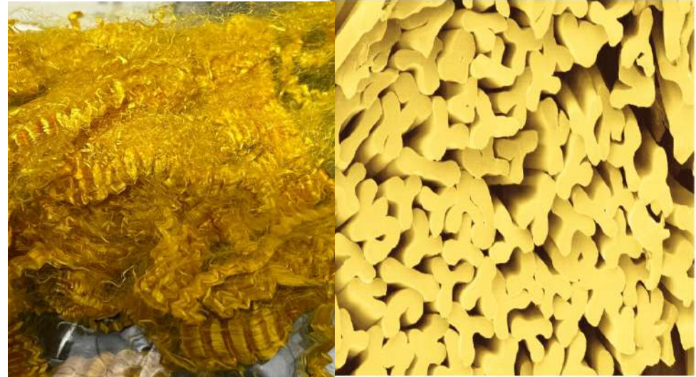
Golden Yellow colour & Multilobal cross-section of P84
