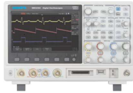
DSO/MSO : SMO2000X Series 70-300MHz, 2/4 Channels with FG RTS 2GSa/s, Memory 140Mpts 16 Channel Logic Input
