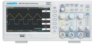
DSO : SMO1000 Series 50 -100MHz Dual Channel RTS 1GSa/s, Memory 2Mpts PC Interfacing Software
