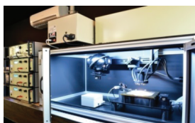
Solar Cell Characterisation System
