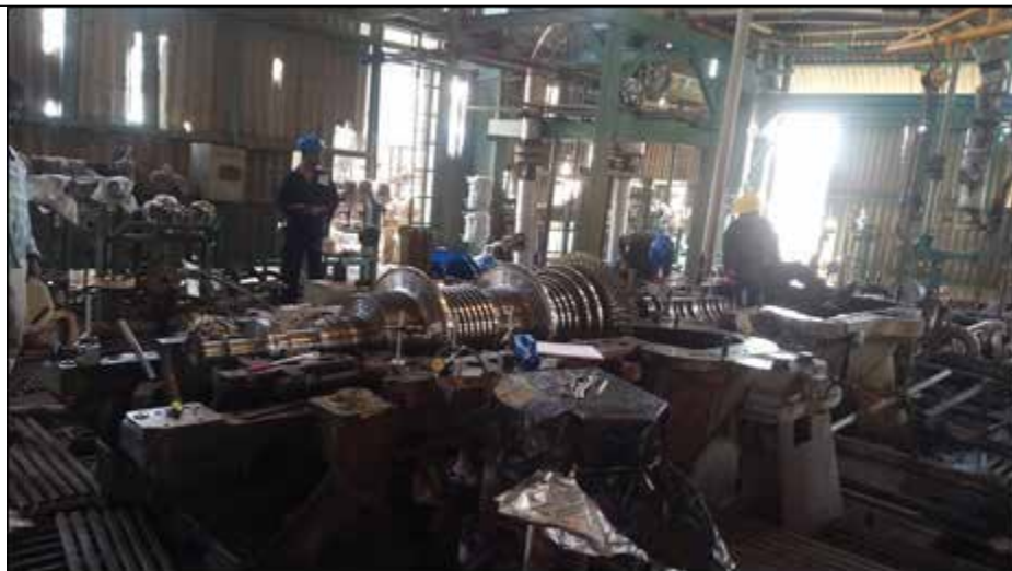
Figure 7. CO 2 compressor with turbine during revamp
